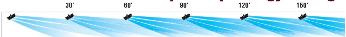
30' apart running at 50% using only 1/4 the energy will provide the near equivalent amount of air as the 60' spacing running at 100%.
