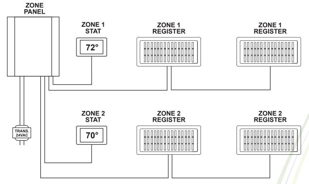
Up to six registers may be connected to a single zone
