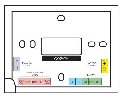
AC / DC The CO2-TH is powered from 12 to 30V AC or DC. If powering with DC +ve is applied to the top terminal
