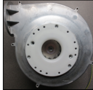
Figure 10 - Installed Adapter Plate
