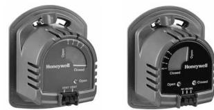
Applications: Replacement motor for EARD ventilation damper Motor Timing: 30 seconds power closed/10 seconds spring return Voltage: 24V Wires to Motor: Terminals: M1-Power; M6 Common; M4 (optional)-LED indication
