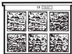
Dirty filter— Needs cleaning
