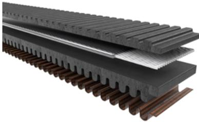
G-Force® C12® belts were the first CVT belt utilizing carbon tensile cord for high modulus and extraordinary strength. This high-performance Neoprene and aramid fiber-loaded rubber belt offers Original Equipment technology. The advanced carbon tensile cords are surrounded by specially formulated adhesion gum to reduce edge cord pullout and increase belt life.
