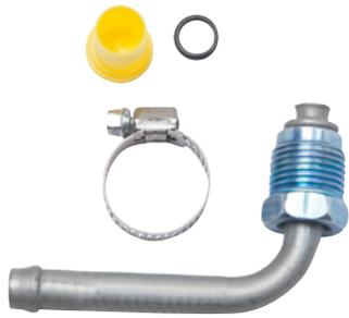
Gates offers a variety of power steering end fittings and adapters for building custom return line assemblies. Simply insert the barbed fitting into the hose and seal with a standard hose clamp. Furnished separately for use with Return Line Power Steering Hose.
