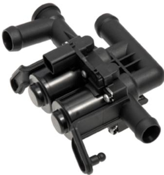
Gates Electric Heater Control Valves are designed to OE specifications in fit, form and performance. They precisely adjust the amount of coolant flowing through the heater core to control the temperature setting in the passenger compartment.
