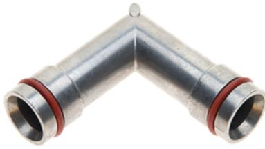
Gates' superior aluminum cooling system connectors carry coolant from the tensioner to the engine with precision-sized ends and high quality EPDM O-rings to create a perfect seal. Developed to replace the failure-prone plastic connectors, which become brittle and crack from high engine heat.
