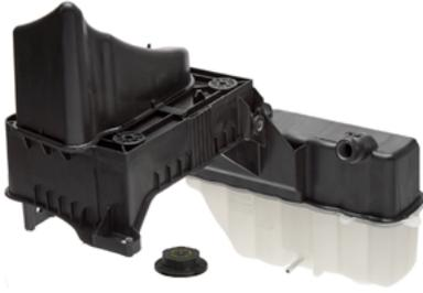
Engine compartment environment, including temperature fluctuations, can damage coolant tanks and reservoirs over time. Gates Coolant Reservoirs are made with high-grade materials to withstand coolant permeation, temperature fluctuations and environmentally-harsh conditions.
