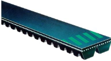
Green Stripe® PowerBand® V-Belts are designed for problematic, heavy-duty, high-vibration applications that require belt sets. The PowerBand technology consists of multiple V-belts joined together by a permanent, high-strength tie band that function as a single unit for improved stability and even load distribution, with a secure strand fit into each pulley groove.
