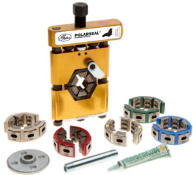
Gates PolarSeal® Portable Crimper is designed for crimping air conditioning assemblies by hand or impact wrench. The PolarSeal Portable Crimper has capability to crimp PolarSeal G45 and G47 couplings and is intended for use with PolarSeal I and PolarSeal II refrigerant hose.
