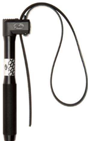
Gates patented strap wrench is specifically designed to grasp and hold automotive SAE Micro-V® belt driven pulleys. The Micro-V wrench grasps the pulley just as an accessory drive belt does when driving an accessory component. Moreover, the action of the tool head pressing back on the component provides unparalleled protection, preventing costly damage. Improve efficiency, reduce component damage and avoid injury by opting for the simple-to-use solution.
