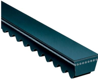
Gates Tri-Power® V-Belts are built for superior performance on heavy-duty drives of classical cross-section. The raw edge construction and special notch design makes the Tri-Power belt especially suited for drives requiring small diameter pulleys and back idlers. The patented ethylene EPDM compound construction allows the belt to resist cracking and handle extreme temperatures.
