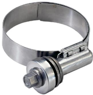
Green Stripe® Constant Tension Clamps provide the reusable, self-adjusting band needed for a dependable seal, even in the coldest conditions. These constant tension clamps feature larger, heavy-gauge, precision-formed spring washers with higher rates of band tension and adjustability for a more dependable seal for use in automotive, truck and bus cooling systems and turbochargers.
