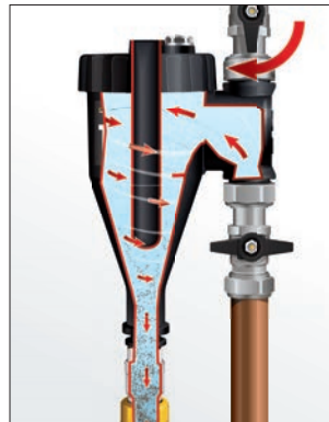
3. Open outlet and drain valves
