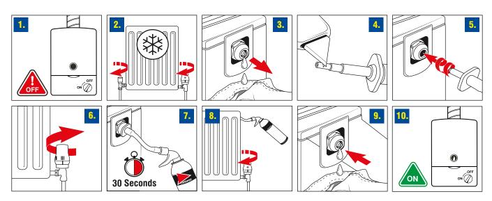
Make sure the system is turned off and allow radiators to cool down (1). Select a radiator and shut both the wheel-head and lock shield valves (2). If a thermostatic radiator valve (TRV) is fitted, close it by turning it to the minimum setting.
