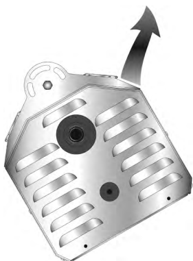
Figure 2.9 • Hot Flue Discharge
