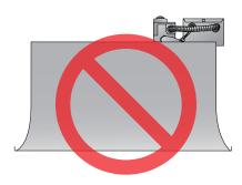
Failure to place control end down will result in damaged controls.
