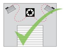
Provide natural or mechanical means to supply and exhaust 4.0 CFM per 1000 BTU/H of gas input.
