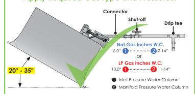
Provide proper gas type (as denoted on heater rating label) and observe minimum and maximum pressures.
