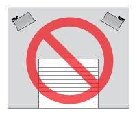
Failure to observe minimum ventilation rates will result in condensation and increased carbon monoxide rates.
