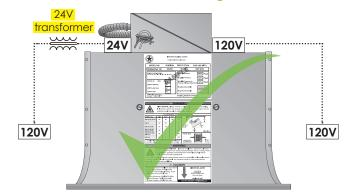
120V systems are installed directly to 120V lines; however, transformers must be used on 24V systems. Install mV systems to mV thermostat as supplied.
