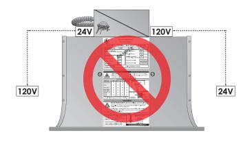
Failure to observe proper voltage will result in damaged controls.
