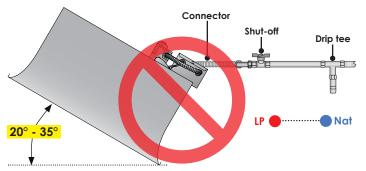
The use of improper gas or improper pressure will result in a fire hazard or improper equipment operation.
