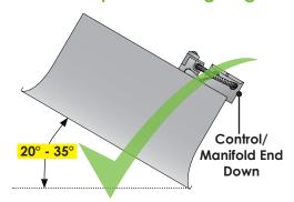
Heater **must be** mounted level side to side and at a **20-35**° angle from horizontal with the control end down.
