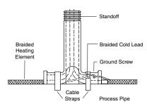
Detail 7. Connect input power wires.
