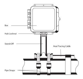
**Detail 3.** Polycarbonate enclosure installed on pipe. (PC1 - Box and hub only. PC2 - includes standoff, pipe straps, hub, ring connector and ground screw).
