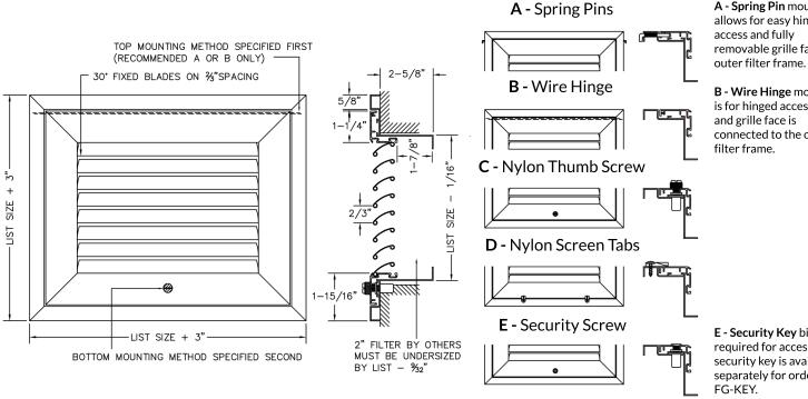
A - Spring Pin mounting allows for easy hinged access and fully removable grille face from
