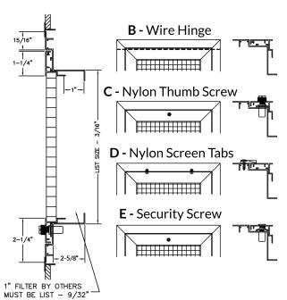
B - Wire Hinge mounting is for hinged access only, and grille face is connected to the outer filter frame.
