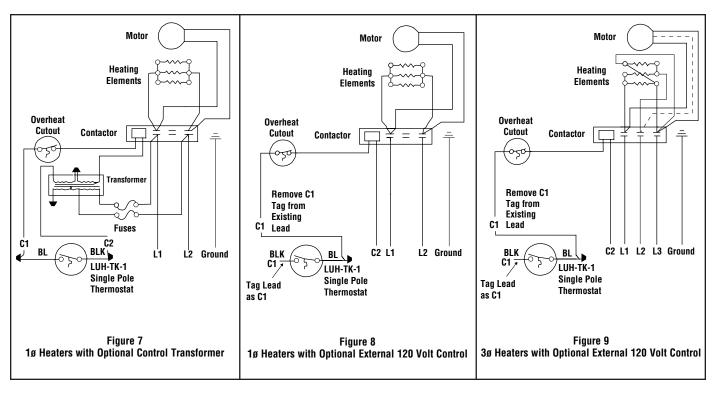
Connect single pole thermostat blue lead (BL) to heater lead C1 and black lead (BLK) to C2 using wire nuts provided.
