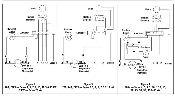
Connect single pole thermostat blue lead (BL) to heater lead C1 and black lead (BLK) to C2 using wire nut provided.
