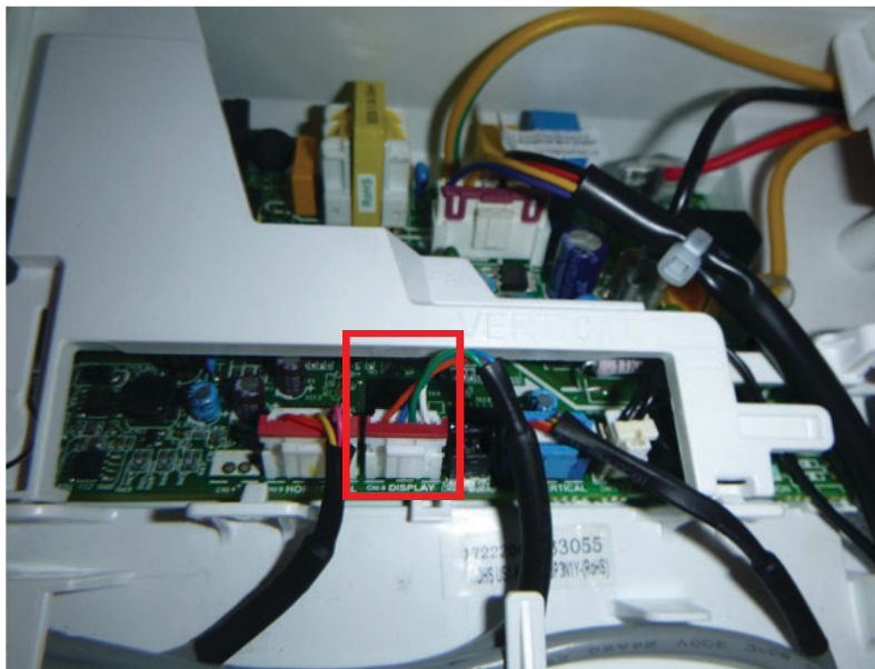
Fig. 13 — Remove the existing harness
