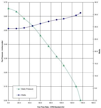
Fan Flow Rate - CFM Standard Air
