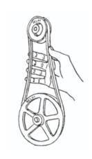
Excessive deflection is an indication that the belt is not tight enough. If not corrected, slippage could cause loss of blower speed and belt failure through wear.
