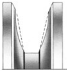
Worn Groove Sidewalls
