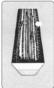
Fabric Worn on Backside
