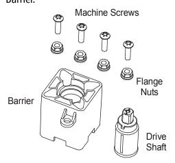
Figure 16: Optional ST2-HT Thermal Barrier
