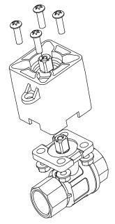
Figure 18: Installing the Barrier
