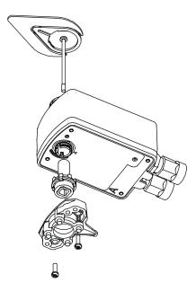
Figure 5: Removing the Linkage
