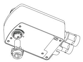
Figure 6: Inserting the Drive Shaft
