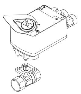
Figure 15: Mount the Actuator
