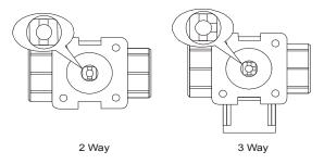
Figure 10: Positioning the Valve Stem
