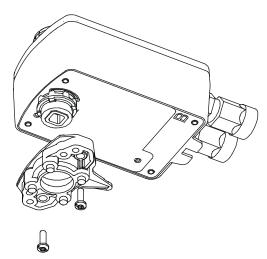
Figure 7: Installing the Linkage
