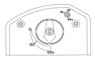
Figure 22: Switch Trip Point Settings
