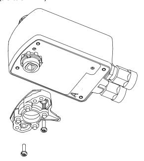
Figure 13: Installing the Linkage
