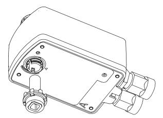
Figure 12: Inserting the Drive Shaft
