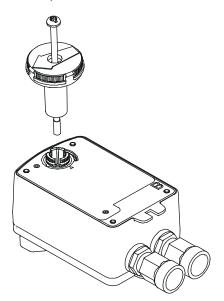
Figure 14: Installing the Fixed Pointer
