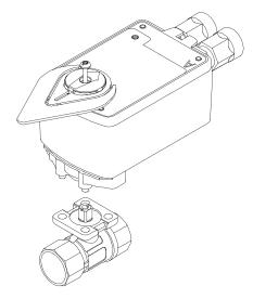
Figure 9: Mount the Actuator
