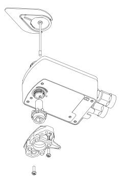
Figure 11: Removing the Linkage
