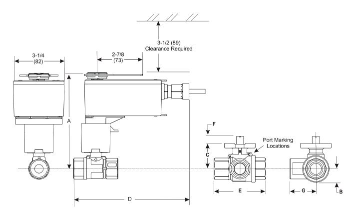
Figure 3: Spring Return VA(M)S24-27 Actuated ST2 Series Ball Valve with Optional ST2-HT Thermal Barrier Installed Dimensions, in. (mm)
