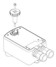
Figure 8: Installing the Fixed Pointer
