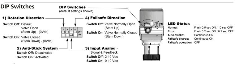
NOTE: <sup>1</sup>The Enerdrive system is a patented method of storing energy (using super capacitors) that is later used to drive the actuator to it failsafe position during a power failure.
