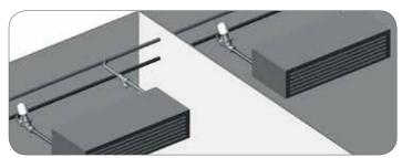
The Simple Set can be mounted in either the supply or the return line. To avoid temperature extremes, it is recommended on the return line. Installation of strainers and isolation ball valves are recommended. The temperature in and about the actuator should not be below 32°F (0°C).
