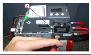
Step 8: Adjust the yellow clutch wheel on the underside of the terminals using a 4 mm wide screwdriver to the 90° position.
