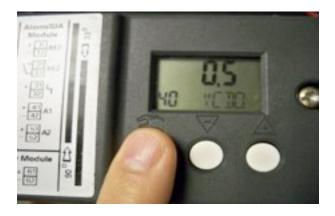
**Step 18:** Change the parameter value to the desired lower limit for tight closing.
