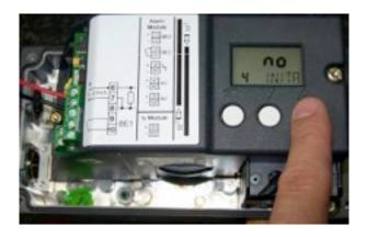
Note: If an error is displayed on your positioner during Run 2, the lower tolerance (down tolerance) of the adjustment wheel has been exceeded. (If no errors are displayed, skip ahead to step 8.)
