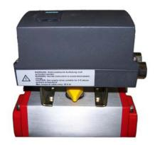
Step 6: Insert the pneumatic fittings on the positioner and actuator before inserting tubing into the outputs of the positioner to the inputs of the actuator.
