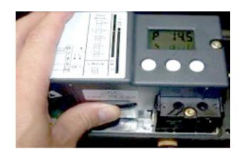
Once the down tolerance error has been corrected, the middle character of the message line will change to an 'O'.
