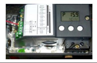
Step 2: Press the Menu Button for >5 seconds to enter into Configuration mode.
