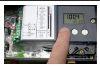
Step 12: While in 'AUTO' mode, test the responsiveness of the device by varying the command signal from 4 mA to 20 mA.
