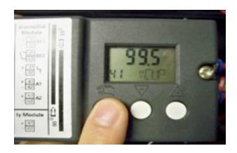
**Step 20:** Change the parameter to the desired upper limit for full open.
