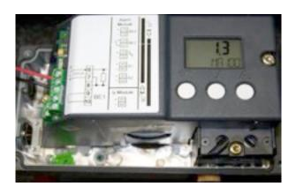
**Step 10:** Use the  $\overline{\nabla}$  or  $\underline{\triangle}$  buttons to manually close or open the valve to ensure that the desired travel limits are being attained.
