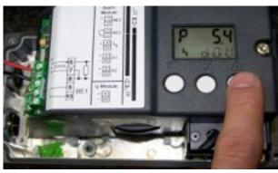
Step 8: Upon successful completion of calibration, the status line will display "FINISH". Press the Menu Button once to exit.
