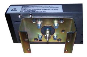
**Step 4:** Position the yellow indicator on the base of the coupler.
