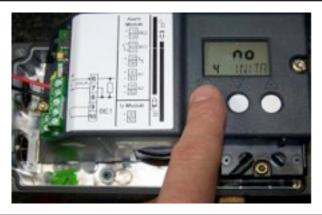
**Step 7**: Hold down the Up Button **≜** until calibration begins (>5 seconds), then release. The device will now progress through 5 "RUNS", completing a series of checks. For more information on the calibration, please refer to the product manual.
