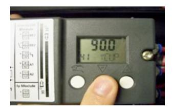
**Step 21:** Exit Configuration mode by pressing the Menu Button for >5 seconds. The device will be in Manual Mode ("MAN').
