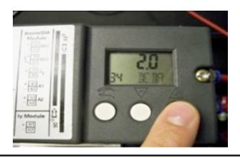
Step 16: Use the Menu Button to scroll to parameter 39 (YCLS). This setting allows users to assign a position where the 6A will default to full open or close. Select 'uP do' by pressing the Up Button. A
