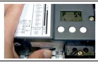
To continue calibration, press the Up Button  $\triangle$  once and release.
