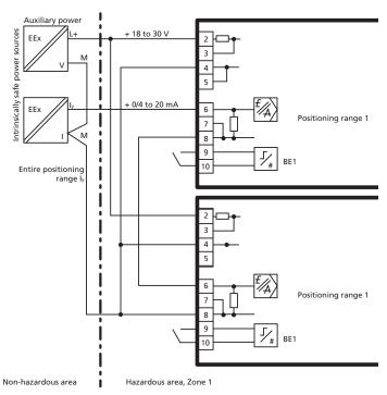
Series connection of 2 positioners, e.g. split range (auxiliary power wired separately), EEx i
