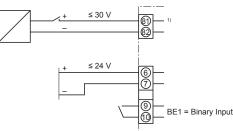
1) Input for safety shutdown (activated using coding jumper)
