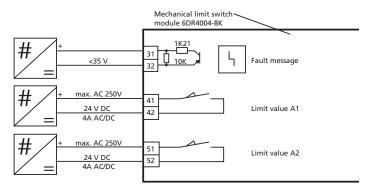
Figure 10. - Mechanical limit switch module 6DR4004-8K, not Ex
