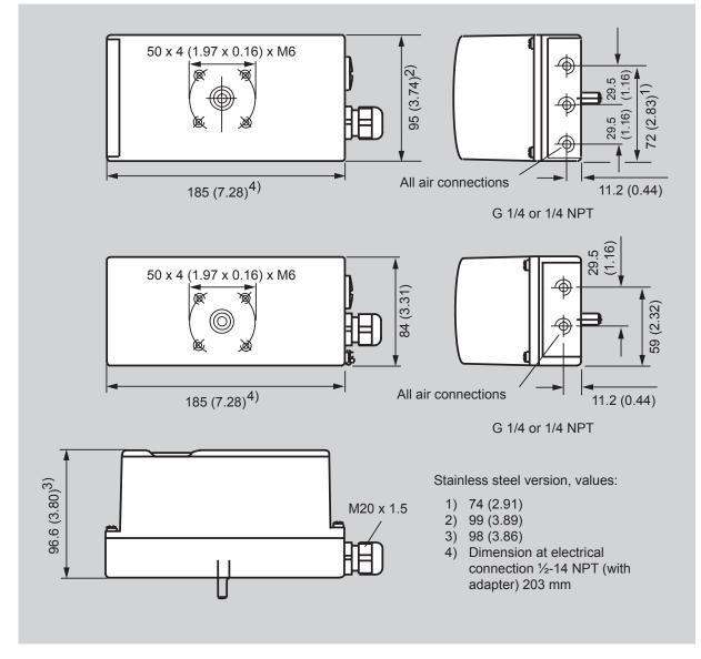
Makrolon and stainless steel enclosure double acting (top), aluminum enclosure single acting (center), Makrolon and aluminum enclosure (bottom), dimensions in mm (inch)
