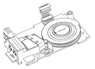
Mechanical Limit Switch Module
