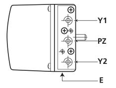
Figure 2. - Pneumatic connection on the standard controller
