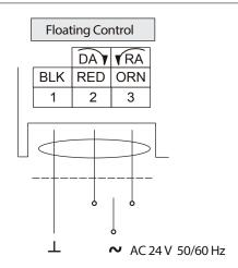
NOTE: To avoid excessive wear or drive time on the motor, use a controller and/or software that provides a time-out function to remove the signal at the end of rotation (stall).
