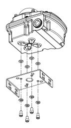
6. Place lock washers on foot plate mounting bolts.
