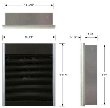
NOTE: \* Will accommodate pneumatic/electric or low-voltage controls commonly used with computerized energy management systems Mounting Limitations: For wall mounting, do not install back box closer than 8 in. from floor or adjacent wall. Do not install heater behind towel rack, behind door, in floor, in closet, in ceiling or where air flow may be obstructed. All controls are concealed behind the front cover making them essentially tamper proof.
