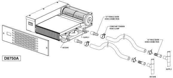
The Twin-Flo III "Easy Connect" flexible hose connection kit allows for easy installation of any 'K' Beacon/Morris Kickspace Heater in new or retro-fit construction situations.
