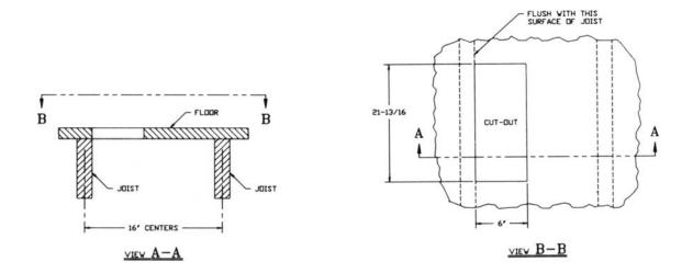
MODEL FK-84 & FK120 FLOOR KIT CUT-OUT ARRANGEMENT PARALLEL TO JOISTS
