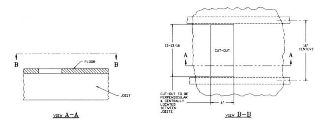
MODEL FK-42 FLOOR KIT CUT-OUT ARRANGEMENT PERPENDICULAR TO JOISTS
