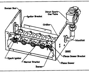
Figure 4 Heat Exchanger Details
