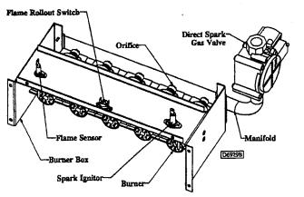
Figure 3 Separated Combustion Tubular 30/75 Unit Heaters
