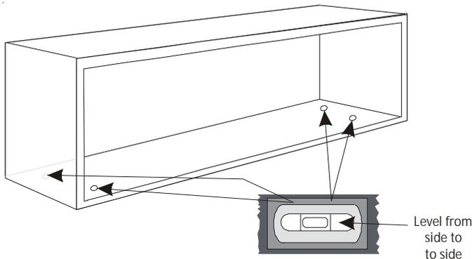
Place level on dimples or next to the dimples in wall sleeves' corners.
