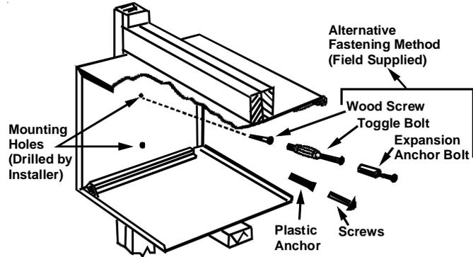
Figure 12 - Wall Sleeve Attachment to Opening
