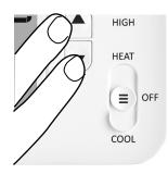
With thermostat powered, move System Mode switch to the OFF position. Press and hold BOTH Up and Down buttons for at least 5 seconds, until the screen changes.
