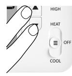
Press BOTH the Up and Down buttons together after last menu item exits the settings menu.
