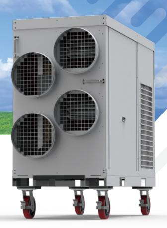
Airrex Portable air conditioner with electric heat operate in air temperatures from 65°to 113°F for cool mode, dehumidification from 86.16 to 124.8(gal/day) and 50°to 81°F for heat mode. These AHSC-140 utilizes eco-friendly 410A refrigerant.
