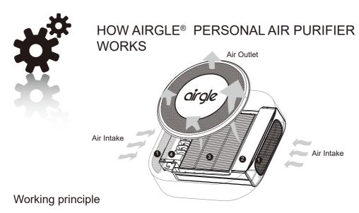
The air enters through the right and left air inlets simultaneously and is rapidly purified. The air, which enters through the right air inlet, passes through pre-filter and carbon filter. The air through the left air inlet is purified through Airgle® Titanium Pro® Module. The air inside the machine is then filtered and purified through cHEPA filter. Lastly, the filtered and clean air is delivered from the face of the machine.
