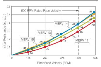
Maximum recommended final resistance for all VariCel® VXL filters is 2 in. w.g.\*
