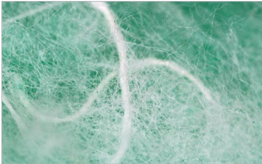
Looking closely at a leading competitor's media, notice the inconsistent fiber sizes and binder that can lead to inconsistent performance and variability.
